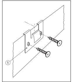
■ Lay the spring clamps supplied ① on the top edge of the cut-out in the positions indicated and secure with 2 screws each.
